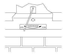
Figure 38 - Opening Vent Damper
